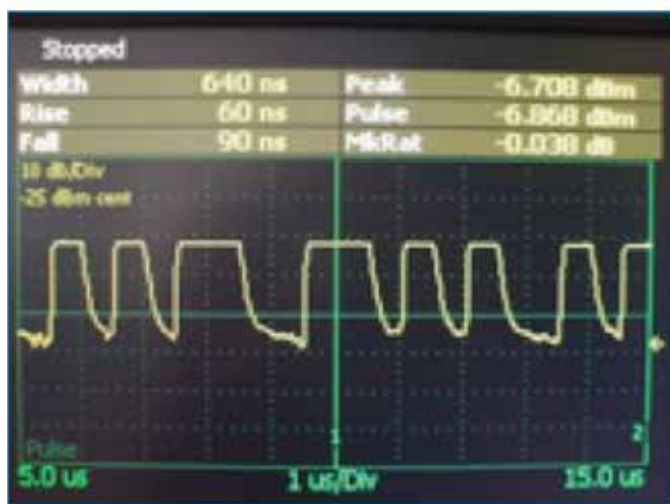
(c) Pulse-train sub-pulse power measurements in pulse mode
