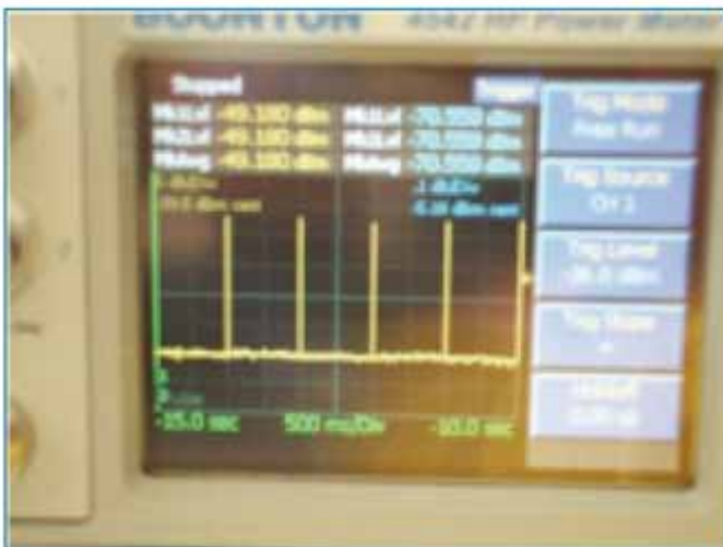
(c) Measuring transponder 'bursts'
