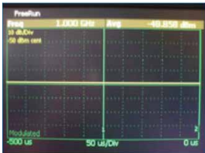
(a) Average power measurement of pulse-
