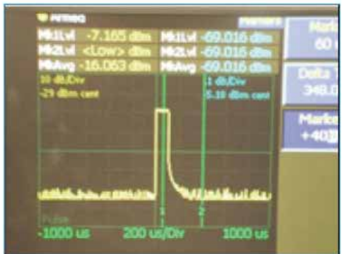
(d) Measuring sub-pulses within a signal burst
