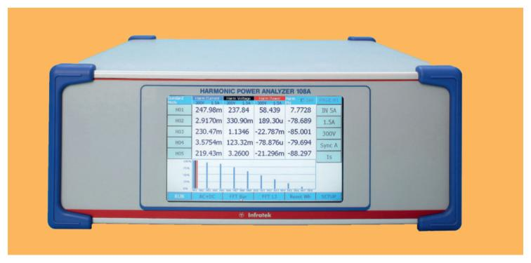
THE MODEL 108A UNIVERSAL HIGH PRECISION POWER ANALYZER MEASURES 280 ELECTRICAL QUANTITIES ON EVERY PHASE. ENERGIES, HARMONICS, MOTOR- AND TRANSFORMER VALUES, POWER SUMS, POWER RATIOS, AND PROCESS INPUTS CAN BE DISPLAYED, OR READ VIA INTERFACE AT ANY TIME.
